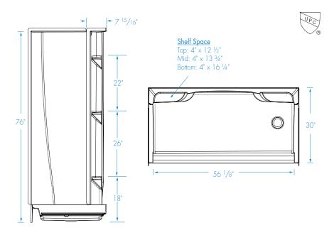
Assembled Model Components: 6030CPANL (Base), 6030CPANR (Base), 6074CBW (Back Wall), 2374CSW (Side Walls)
