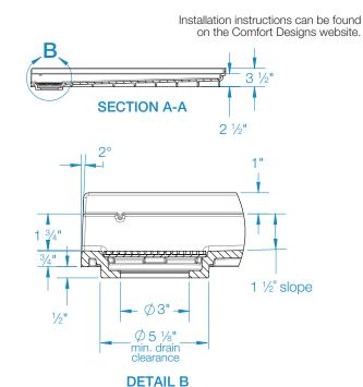
$FEATURES \ \ \, \text{Dimensional Tolerance} \,\, \pm \,\, \text{\%"}. \, \text{Dimensions needed for site preparation should be measured from the unit. Comfort Designs assumes no responsibility for preparatory work.}$
