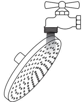
Reinstall the showerhead. Turn on the water and allow the showerhead to flush for at least one minute.
