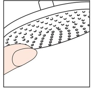
If scale deposits are noticed on the spray face, pour about 3/4" of a commercial scale remover, such as Lime-Away™ or CLR™, into a shallow dish. Dilute the remover according to the label instructions.
