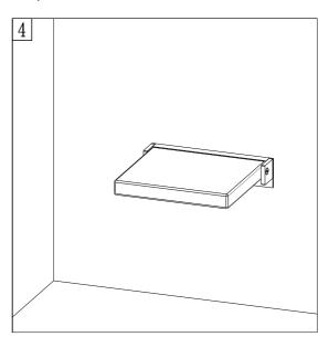
Fasten the PU seat pad on the bracket by 2 pcs screws and ensure the seat pad can be moved along guide channel smoothly,then these screws can be locked.
