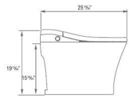
This toilet is designed to rough-in at a minimum dimension of (12") from finished wall to C/L of outlet. Supply not included with fixture and must be ordered separately.
