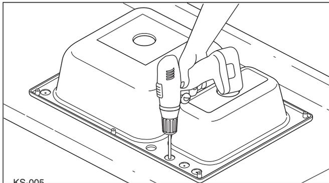
7. Drill the additional hole(s), using the  $1/4"$  pilot hole for a guide, with a  $1-3/8"$  hole saw.
