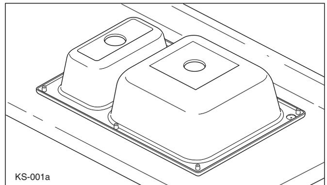
2. Trace a pencil line around the outside edge of the sink and remove the sink from the countertop.
