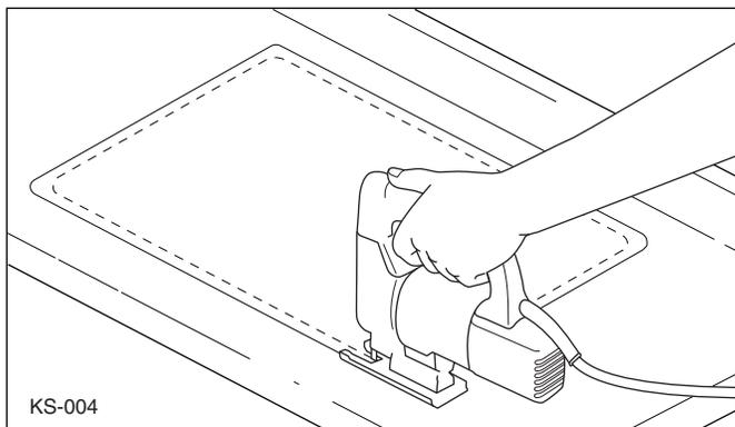
**Note:** All Swanstone sinks are manufactured with one predrilled hole. Optional locations for additional holes are located on the underside of the sink using marks which are cast into the sink. Follow Steps 6 and 7 for drilling additional holes to meet the requirements of the sink faucet or other accessories.
