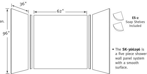
Designed to fit base areas 36" deep or smaller x 62" wide x 96" high or smaller (914 mm x 1575 mm x 2438 mm)
