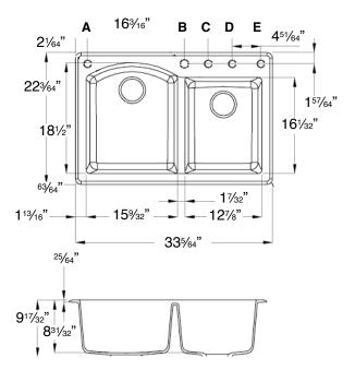
IMPORTANT: Circle Letter(s) above to indicate location(s) for faucet hole drillings (there is a 4" spread between hole locations B,C,D. There is a 16<sup>3</sup>/<sub>16</sub>" spread between hole locations A and B and a 4<sup>51</sup>/<sub>64</sub>" spread between D and E).
