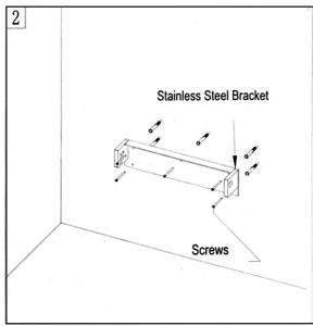
Fix the position of mounting holes on wall depend on the actual dimension of Stainless Steel Brackets(a total of 5holes)
