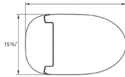
This toilet is designed to rough-in at a minimum dimension of (12") from finished wall to C/L of outlet. Supply not included with fixture and must be ordered separately.
