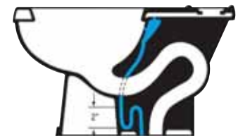
SIDE CUT-A-WAY SHOWING SECONDARY TRAP HT
