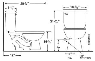
This toilet is designed to rough-in at a minimum dimension of 305mm (12") from finished wall to C/L of outlet. Supply not included with fixture and must be ordered separately.
