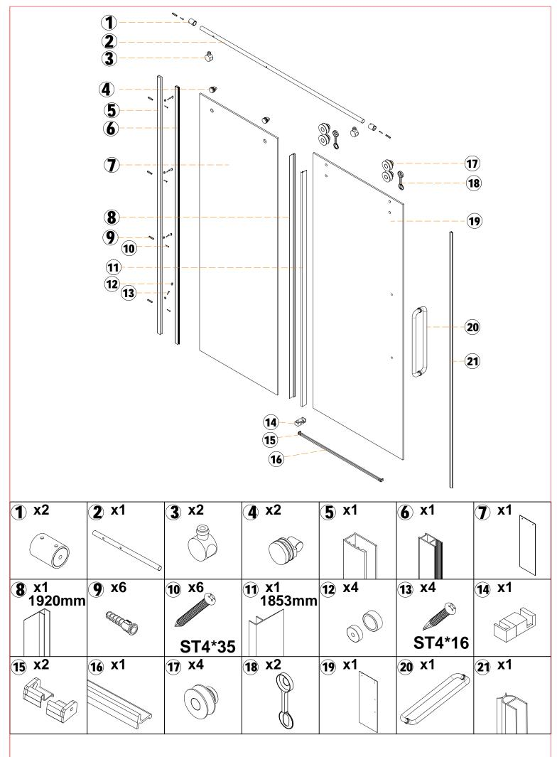
Place the aluminum wall profile on the mounting position and draw the location of the hole. Use an 6 drill bit to drill the made position, Insert wall anchor into the drilled holes and lock them on the wall with (10)**5** Ø 6 ST4\*35
