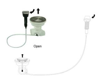
Turn the remote knob clockwise to open the drain.
