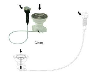
Turn the remote knob counter-closkwise to close the drain.
