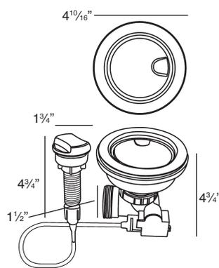
Turn the remote knob to open and close drain. Water drains easily when cover is in place. Cover flips up with easy touch. Polypropylene housing. Fits standard 3 1/2" opening. 1 3/8" hole required in countertop for remote installation. Remote cable 25 1/2" L.
