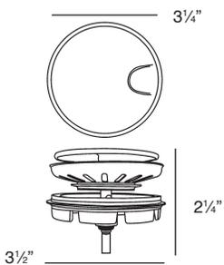
Water drains easily when cover is in place. Cover flips up with easy touch. Polypropylene housing. Top mount installation for 3 1/2" opening.
