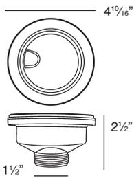
Water drains easily when cover is in place. Cover flips up with easy touch. Polypropylene housing. Fits standard 3 1/2" opening.
