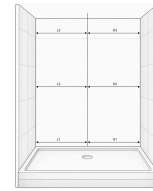
Fig. 8: Measure L and R at three heights
