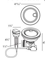
Turn the remote knob to open and close drain. Water drains easily when cover is in place. Cover flips up with easy touch. Polypropylene housing. Fits standard 3½" opening. 13/8" hole required in countertop for remote installation. Remote 43/4" cable 251/2" L.
