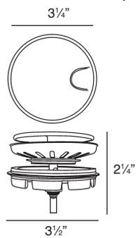
Water drains easily when cover is in place. Cover flips up with easy touch. Polypropylene housing. Top mount installation for 3½" opening.
