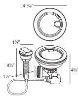
Turn the remote knob to open and close drain. Water drains easily when cover is in place. Cover flips up with easy touch. Polypropylene housing. Fits standard 3½" opening. 1¾" hole required in countertop for remote installation. Remote cable 25½" L.
