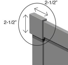
The solid surface corner blocks (set of 2) used at the top outside corners of the walls for a decorative finished appearance.
