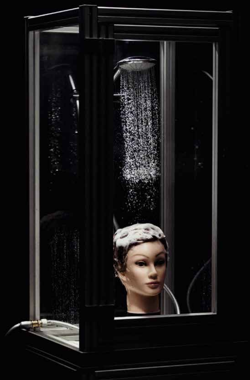
Bensing's shower lab examines shower head spray patterns, analyzing how they can be optimized to save water and increase efficiency.
