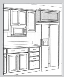
Refrigerator Wall Cabinets range from 12" to 24" high and are 24" deep.
