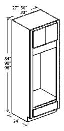
Oven Opening: Height = 47-1/4" Width = 6" less than cabinet width (trimmable)
