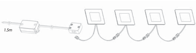
Image shows how this product is wired to a driver Each cable on the product is 1m
