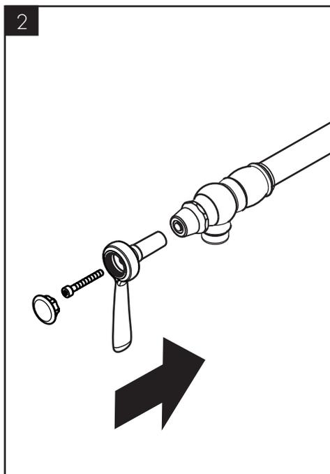
Install the handle screw and screw cover.
