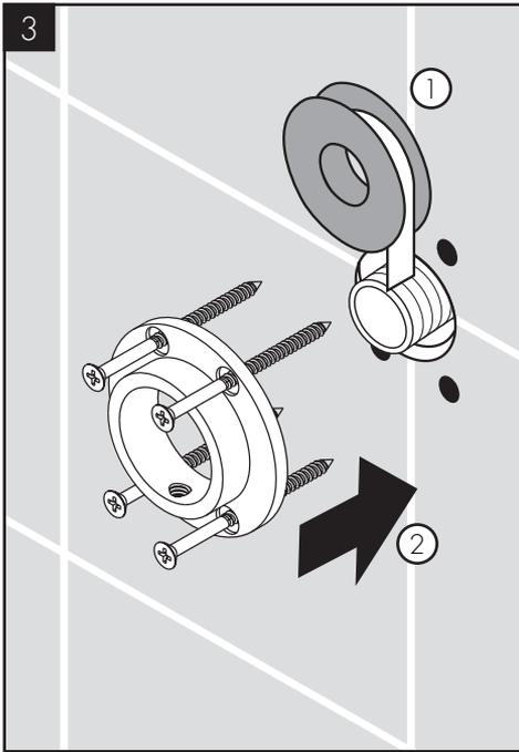
Wrap the threads on the nipple with plumber's tape.
