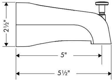
**Read the installation instructions for the shower valve before installing the #06501000 tub spout with diverter. Some shower valves cannot be used in combination with diverter tub spouts.**
