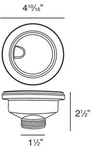
Water drains easily when cover is in place. Cover flips up with easy touch. Polypropylene housing. Fits standard 3 1/2" opening.
